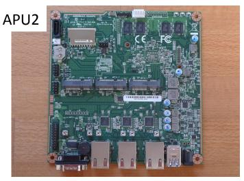
CPU AMD Geode Embedded GX-412TC, 1GHz Quad Core RAM 2GB or 4GB
