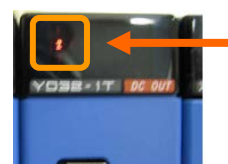
Figure 4: front-panel indicator of a Dout module
