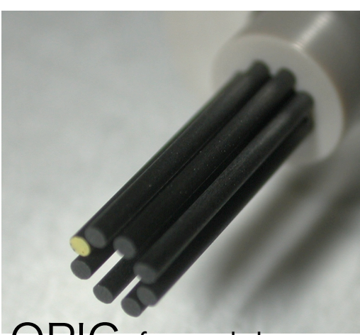
OPIG rf octopole beam guide made of CFRP
