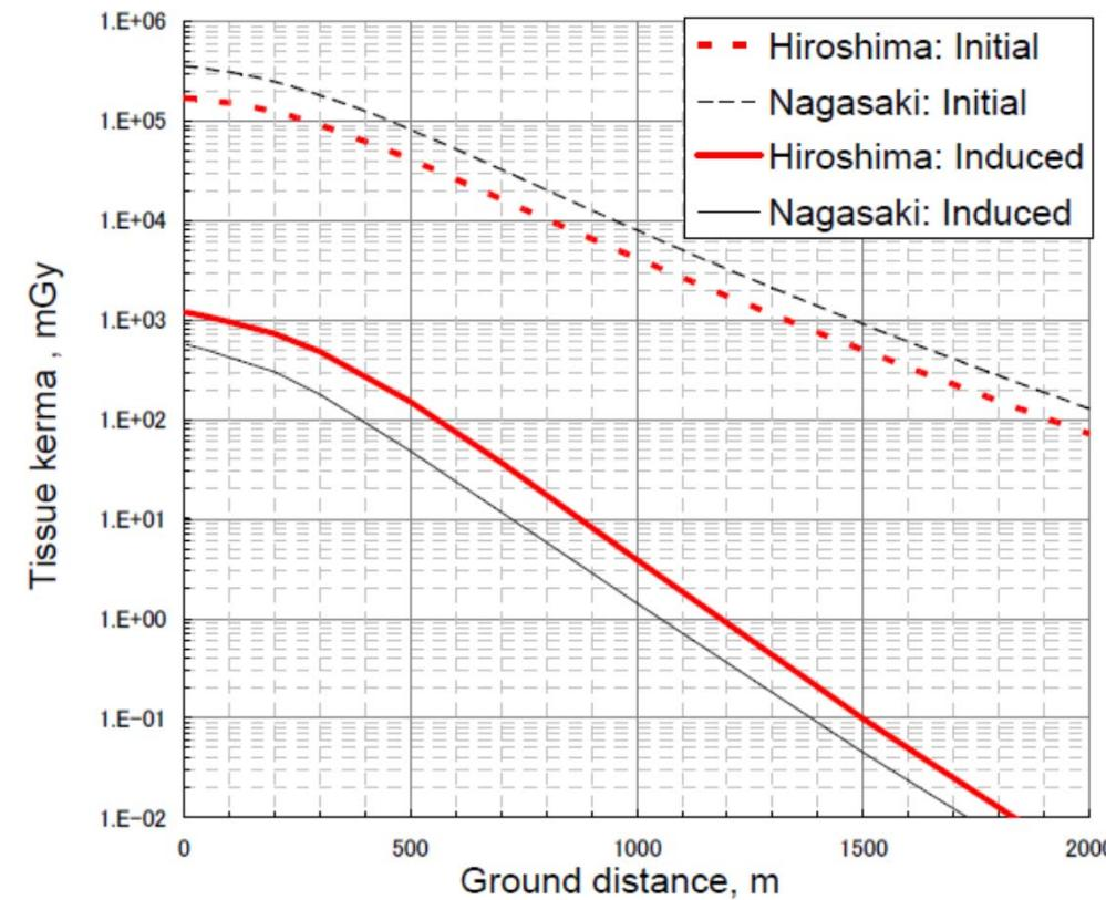
Initial radiation from the explosion vs neutron-induced radiation from the ground (infinite cumulative after the explosion)
