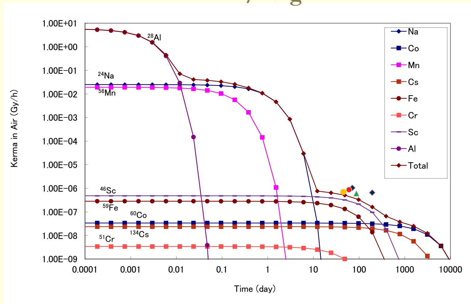
Radiation exposure rate after the bombing due to induced radionuclides in the ground: hypocenter in Hiroshima
