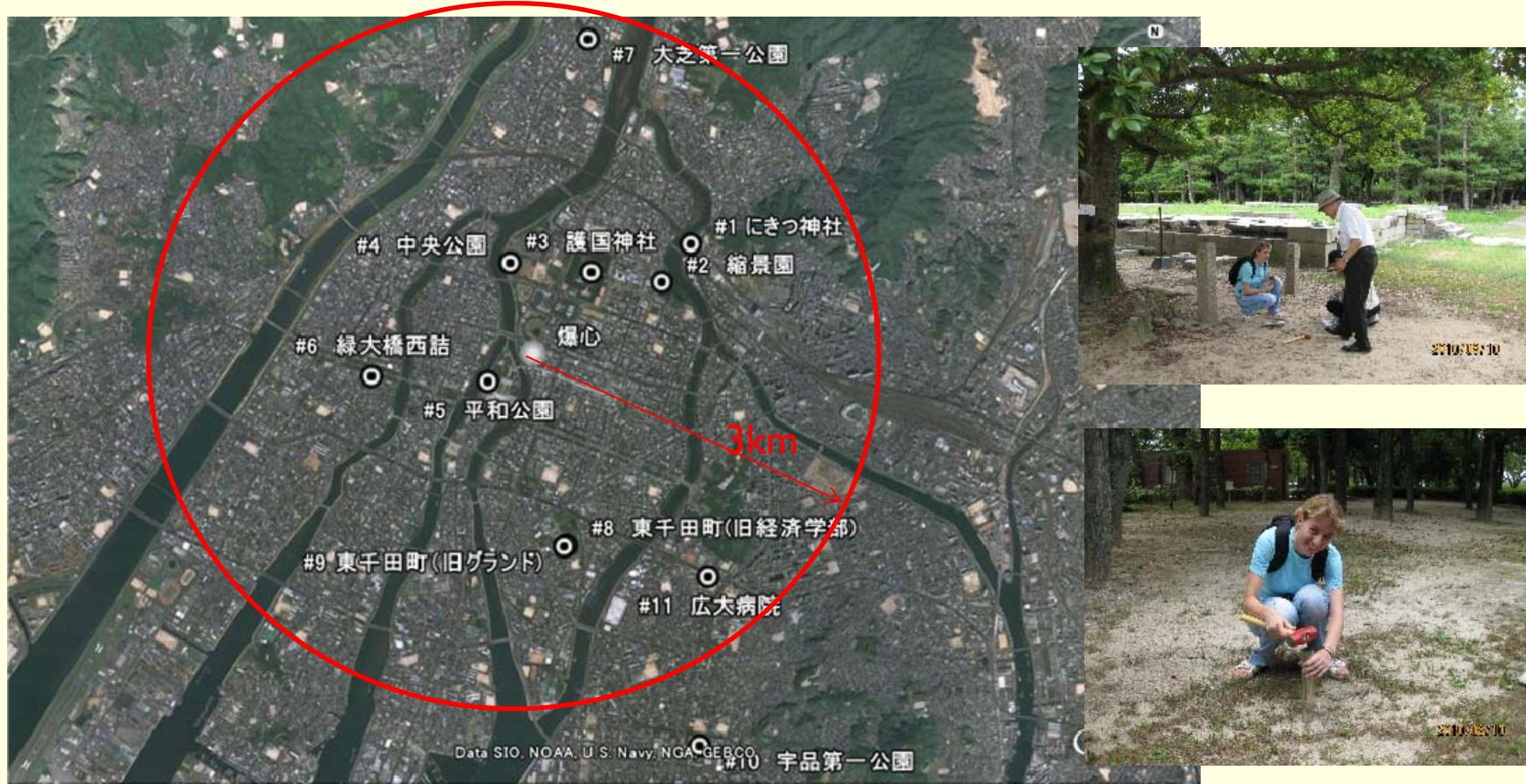
11 soil samples were taken in Hiroshima in August, 2010 for neutron-activation analysis at KUR.
