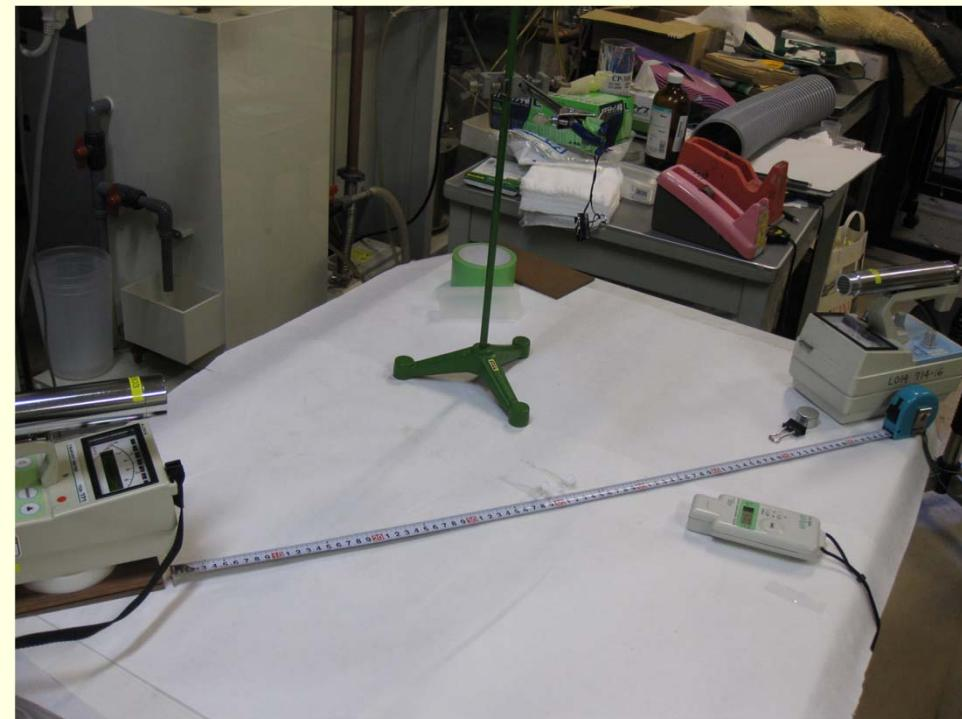
Experiment to observe the initial attenuation of activated soil for the first minutes after 10 sec irradiation by KUR, using GM and NAI survey meters.
