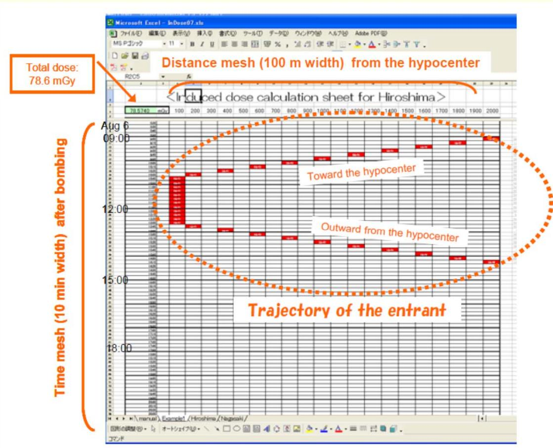
Excel tool calculating external radiation due to neutron-induced radionuclides in the ground.
