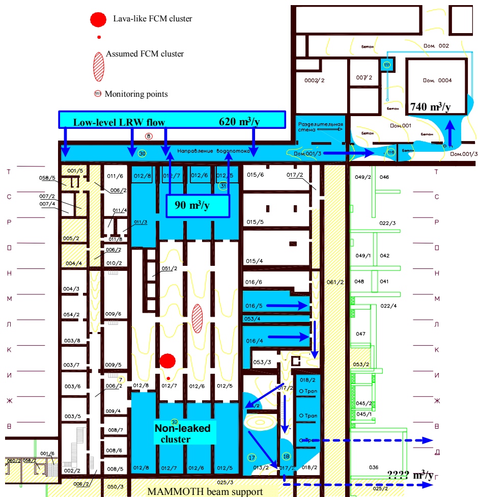
Figure 8 - SO LRW clusters and flows in pressure suppression pool (mark -0.650) and RDAS unit premises (mark -2.600 and +6.000)
