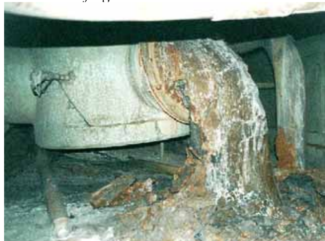
Figure 6 – Lava in steam discharge valve of SDC
