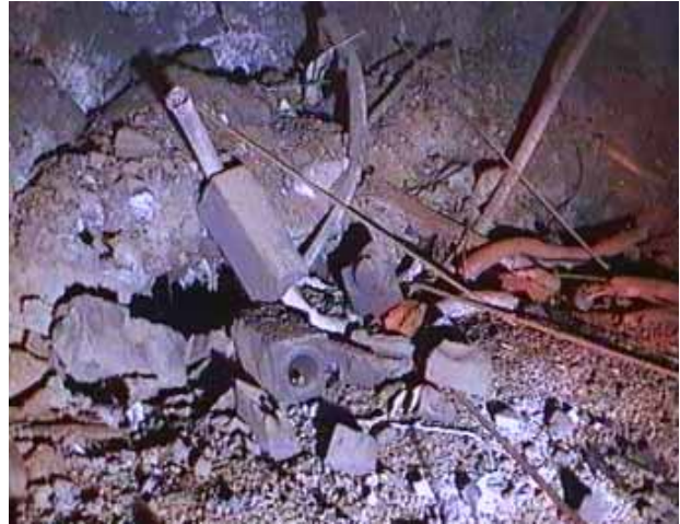
Figure 5 – Premises 305/2. Southeast sector. Active core fragments
