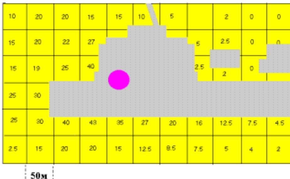
Fig. 5. The nuclear fuel distribution, released to the Unit-4 site at the accident (in kg on site  $50 \times 50$  m<sup>2</sup>).
