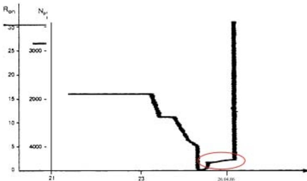
**Fig.2. The change of the power ( $N_p$ ) of the Unit-4 reactor in the diapason of the time from 23 h 00 min 25.04.1986 to the official moment of the accident 26.04.1986 .(The magnified part of the curve in Fig. 1). The unabated increasing of the reactor power calls attention.**
