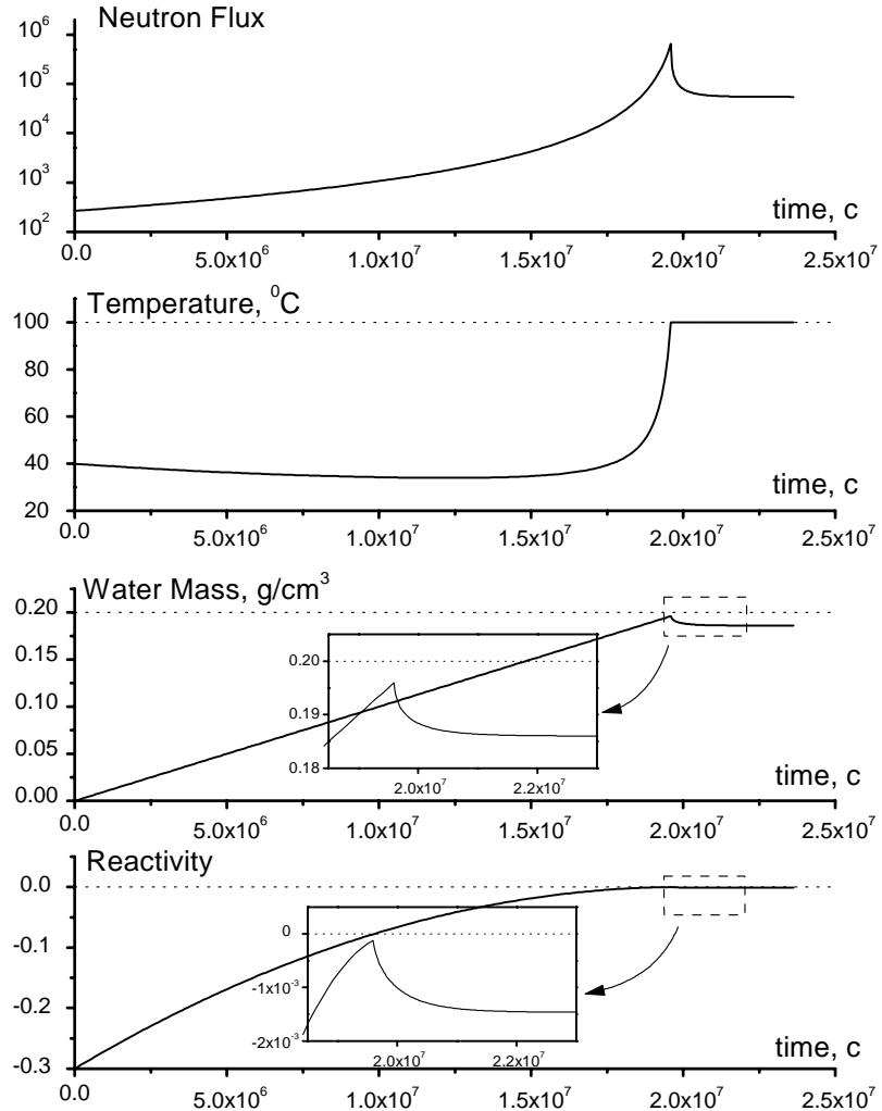
**Fig. 8. Mode of an aperiodic subcritical burst.**
