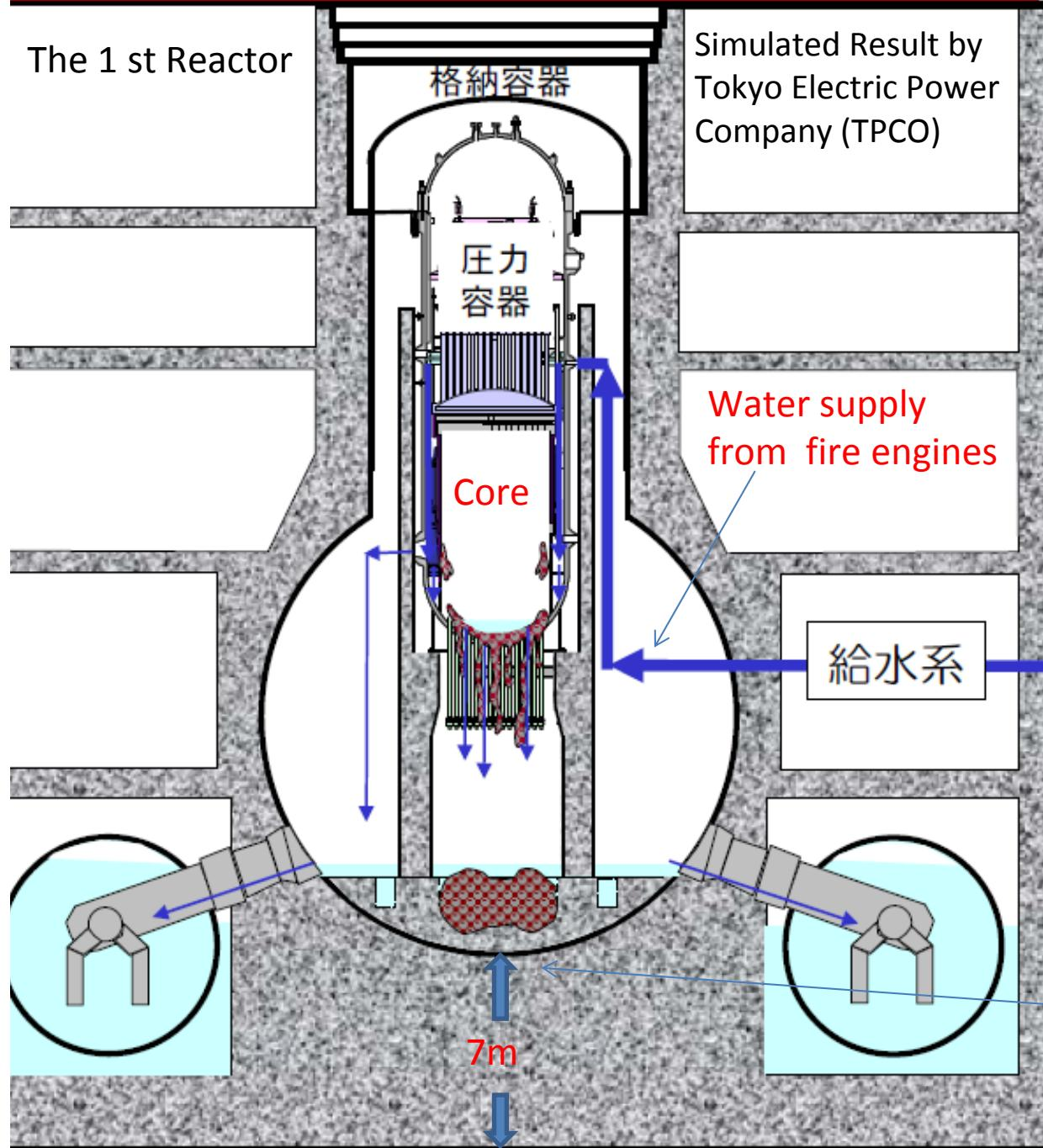
Fig.8 Present status of the 1st reactor molten core by simulations of (TPCO).
