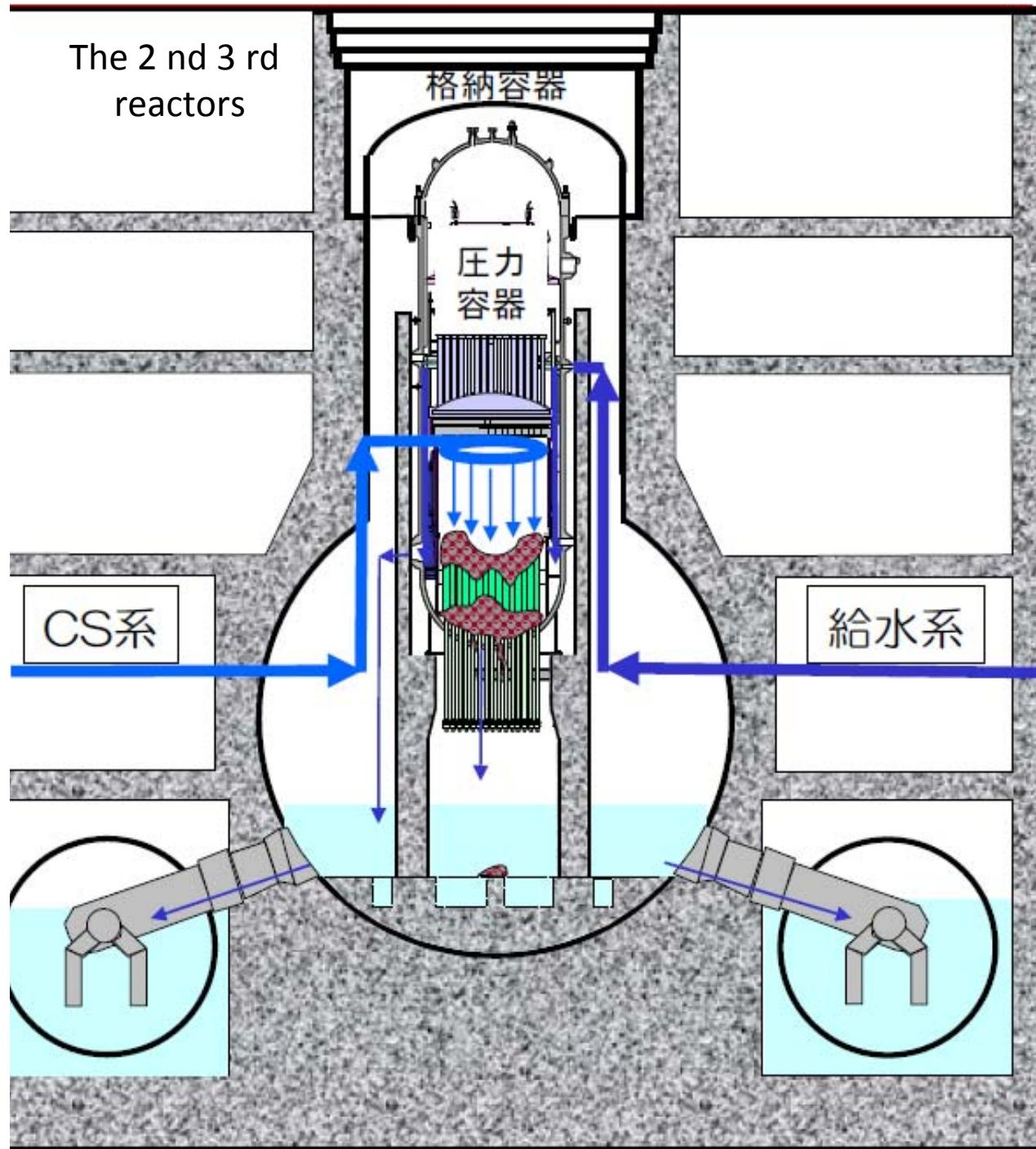
Fig. 9 TEPCO estimates that 60 % of the molten core fell down on the base of PCV in the maximum.
