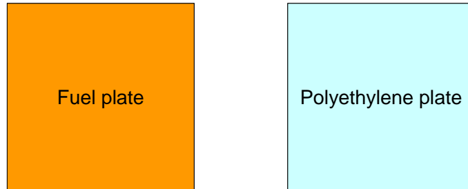
Fig. 1-3 Description of fuel (HEU; 2"×2") and polyethylene plates (2"×2")
