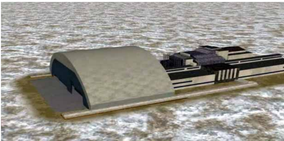
Figure 26. Modeling of arched structure's pushing process to «Shelter» object.
