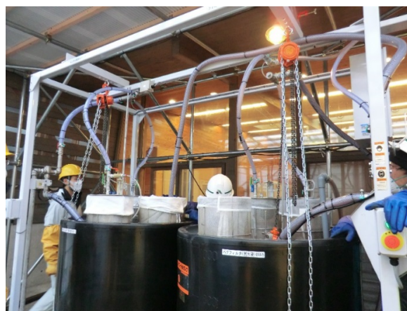
Fig.1 Out view of water contamination system made of two water tanks (black tanks) and control system.
