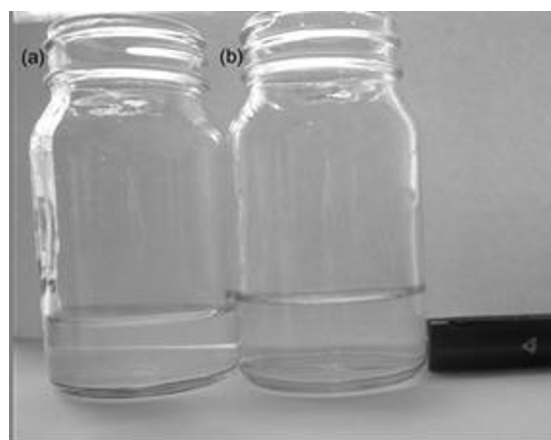
Figure 1 Photographs of aqueous sodium metasilicate irradiated by a green laser (Wavelength: 532nm) after storage for one-half year. The metasilicate was dissolved in water (a) without crushing, and (b) with crushing. The black object in the lower right corner is the green laser. 1)
