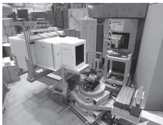
Fig. 1. The compact versatile neutron diffractometer located at the B-3 beam port of KUR.
