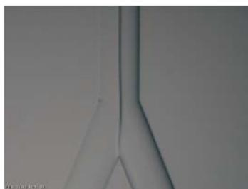
Fig 3. Laminar flow was formed by two solvents of aqueous(Right)-organic(Left) multiphase flow.
