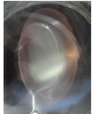
Fig. 2. Solid hydrogen in the target cell
