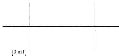
Fig. 2 ESR spectrum of the hydrogen atom encapsulated in the D4R cage after \gamma -ray irradiation.
