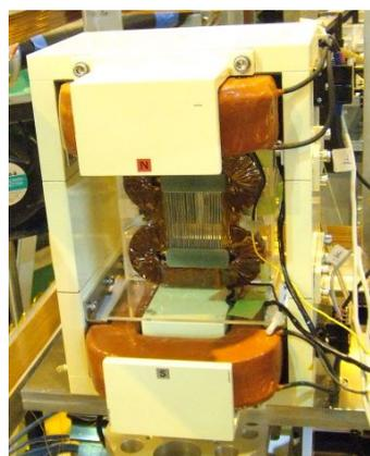
Fig. 1. RSF with dipole magnet with iron pole.
