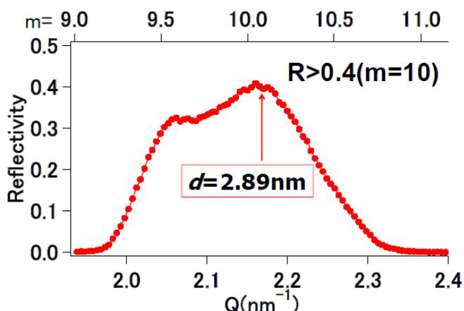
Fig.2. Measured reflectivity by m > 10 wide-band monochromator which consist of four mirrors (8 multilayers).
