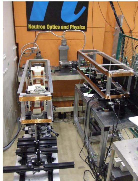
Fig. 1. MIEZE spectrometer in the beam line BL05 NOP in MLF at J-PARC (left side).
