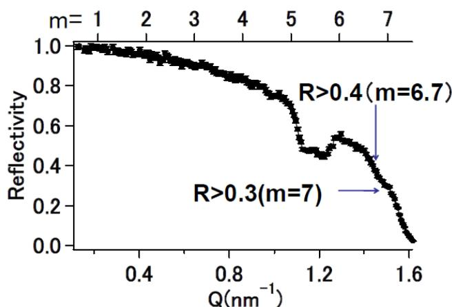
Fig. 1. Measured reflectivity by m=7 NiC/Ti supermirror which consist of stacking two mirrors (4 multilayers).
