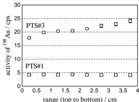
Fig. 2. The activity variation of <sup>198</sup>Au produced at PTS#1 and PTS#3 in HANARO.
