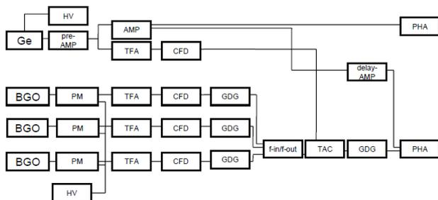
Fig. 1. Anti-coincidence system in KURRI-PGA.
