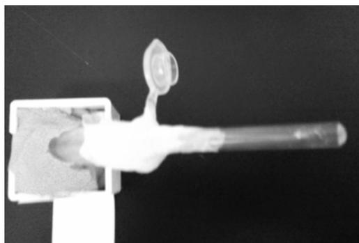
Fig. 1. The photograph of the H/D exchange system of the undeuterated RNase A crystal.
