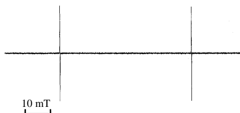
Fig. 2. ESR spectrum of hydrogen atom encapsulated in D4R cage of irradiated Q_8M_8 .
