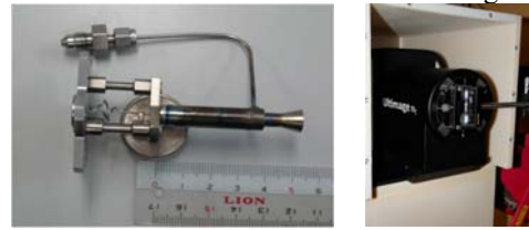
Fig. 2. Shooting sample of the neutron radiography.
