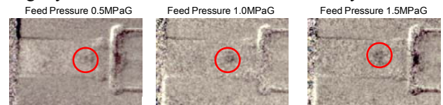
Fig. 3. Images of hydrazine injection.
