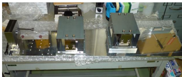
Fig. 1. Photograph of two bending magnets comprised of permanent magnets.
