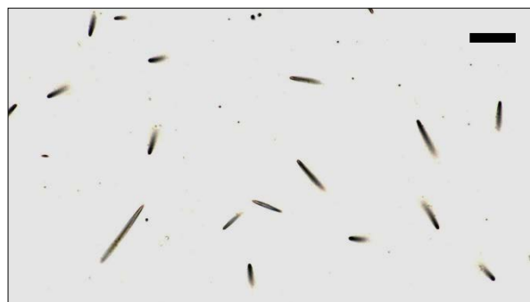
Fig.2. Induced tracks on polycarbonate film Scale bar: 10 \mu\text{m}
