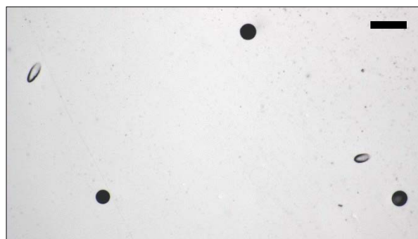
Fig.1. Spontaneous fission tracks in moldavite Scale bar: 10 \mu\text{m}
