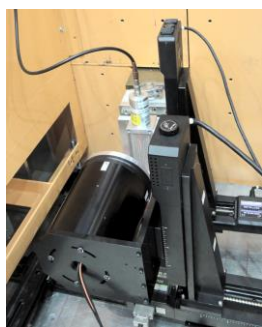
Fig. 1 The beam divergence measurement system on BL05.
