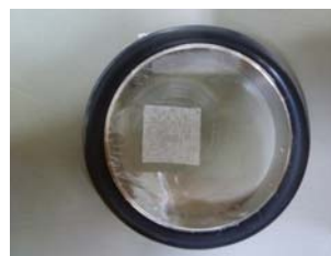
Fig.1 The photograph of the sample. The paper tissue soaked in water was put between two sheets of polyvinylidene chloride film.
