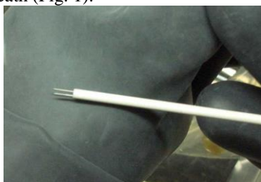
Fig.1 Working and counter electrodes (0.6 mmφ tungsten wire).
