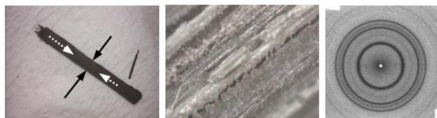
Fig. Macroscopic appearance(a: left), optical microscope image (b: center, x40) and WAXD pattern (c: right) of bamboo matrix prepared by "secondary doping" with  $Ag^+$  following "iodine doping".
