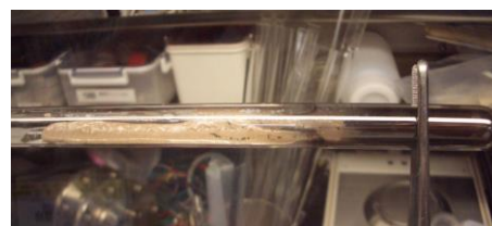
Fig. 2. Deposit formed at the surface of the quartz cell after the electrolysis applied at -1 V for 13 hours.
