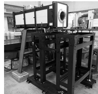
Fig. 1. A neutron transport tube. A neutron detector was placed on the table.
