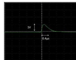
Fig.2 A pulse from B-10+ detector using a charge amplifier
