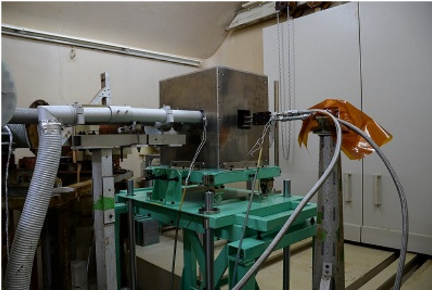
Fig.1 New neutron source installed in KURRI-LINAC
