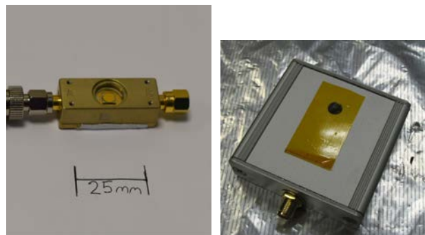
Fig. 1 Diamond detector (left: S1, right: C1,C2)
