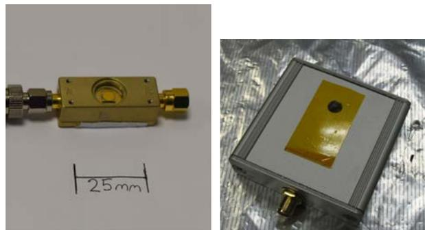
Fig. 1 Diamond detector (left: S1, right: C1,C2)
