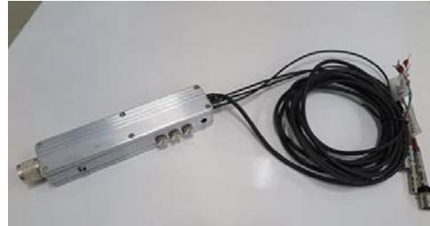
Fig. 1 Amplifier for a neutron detector
