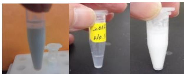
Figure 1. Formulation of <sup>10</sup>BPA WOW emulsion. Left: Precipitate, Center: Supernatant, Right: Mix
