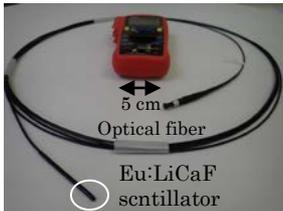
Fig. 1 Detector coupled with the optical fiber.
