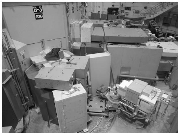
Fig. 1. The compact multipurpose neutron diffractometer, installed at the B-3 beam port of KUR.
