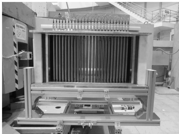
Fig. 2. Twenty-five <sup>3</sup>He tube detectors (1/2 inch in diameter) on the detector bank.
