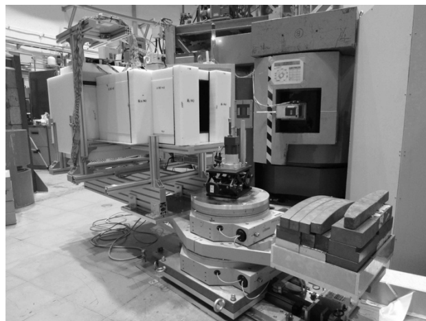
Fig. 1. The versatile compact neutron diffractometer (VCND), installed at the B-3 beam port of KUR.
