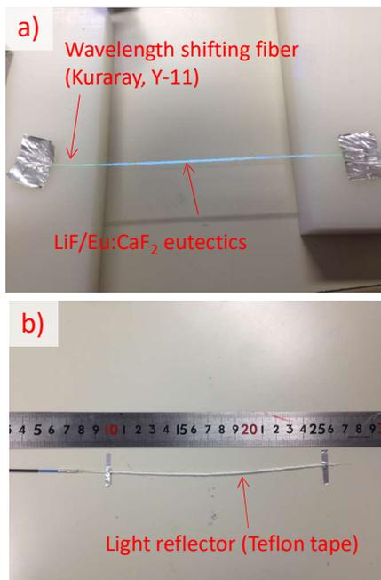
Fig. 1 Photograph of the fabricated new detector. a) Small LiF/Eu:CaF<sub>2</sub> eutectics scintillators were dispersed on side surface of WLSF. b) After wrapped by Teflon tape reflector.
