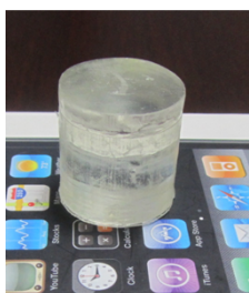
Fig. 1. Appearance of iodine-added plastic scintillator. (diameter : 25 mm, height : 25 mm)
