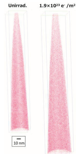
Fig. 2. Atom maps of Re for W-5%Re alloy before and after electron-irradiation.
