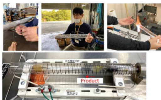
Fig. 1. Building the electric furnace for the sublimation purification method.
