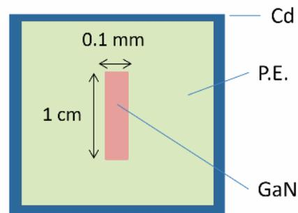
Fig. 1. Calculation model of epi-thermal neutron detector.
