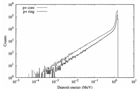
Fig. 2. Deposit energy of 1.47 MeV alpha particles inside the SV for p+ core and p+ ring.
