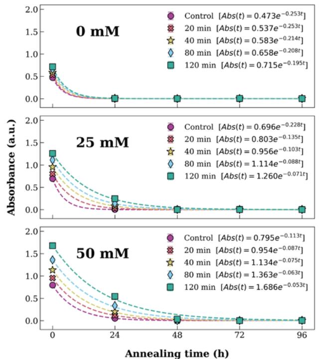
**Fig. 2** Absorbance decay plots of the gel samples with different boric acid concentrations annealed at 50°C. All data sets were fitted with an exponential decay function:  $A(t) = A_0 * \exp(-kt)$ .
