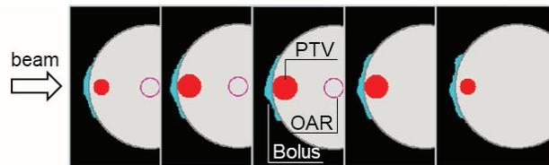
Fig. 1. Phantom geometry with the optimized bolus.
