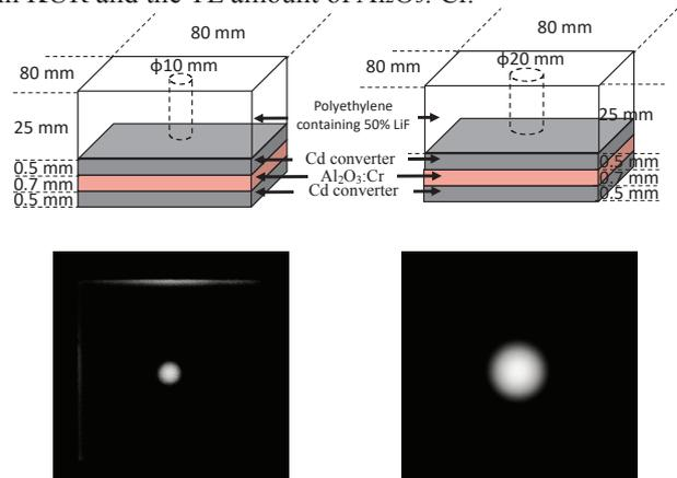
Fig.2 Upper: Arrangement of TL slabs (Al<sub>2</sub>O<sub>3</sub>: Cr using Cd converter) irradiation arrangement for TL imaging. Lower: TL image of the slab.
