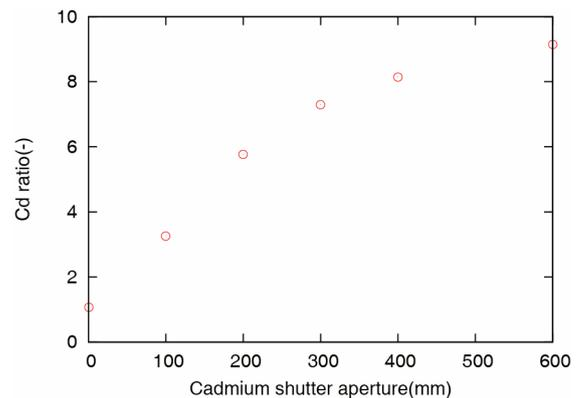
Fig. 2. Relationship between the cadmium ratio and the aperture size of cadmium filter.
