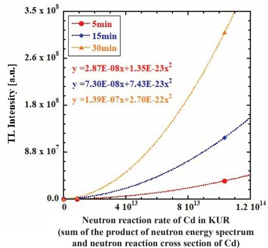
Fig.1 relationship between the neutron reaction rate of Cd in KUR and the TL amount of Al<sub>2</sub>O<sub>3</sub>: Cr.
