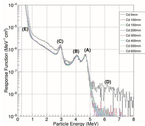
**Figure 1. Pulse heights of neutron detector, which is consisted of thin Si sensor and ultra-thin LiF neutron converter, measuring BNCT neutron beam. Thermal neutron fluxes were changed by opening the Cd aperture window.**
