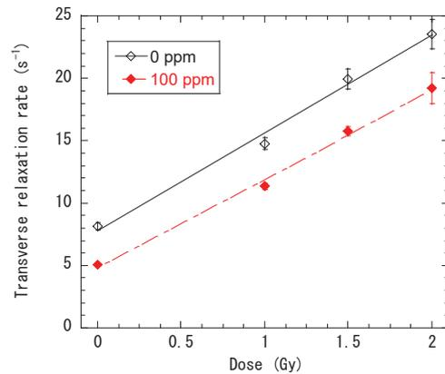
Fig. 1 Response of the gel detector to <sup>60</sup>Co gamma rays.
