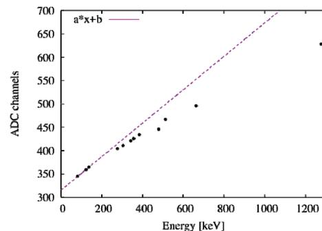
Fig. 1. Relationship between ADC channels and gamma ray energy.
