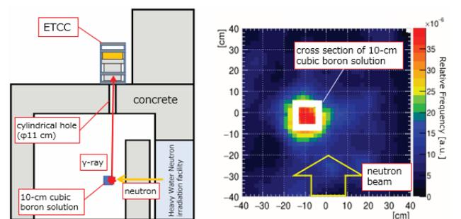
**Fig. 2. Schematic view and obtained image of 478 keV prompt gamma rays from 10-cm cubic boron solution**
