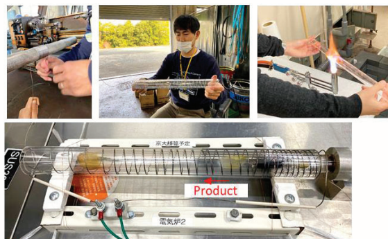
Figure 2 Purification methods tested in this study
