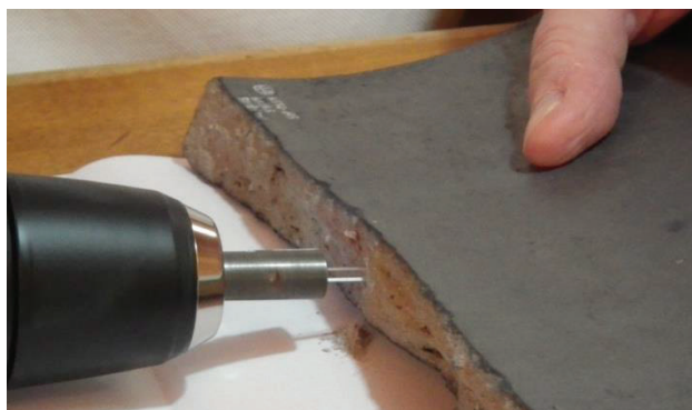
Fig. 1 Sampling with drilling on the broken side of the excavated roof-tile in the site in KU campus, the other side of which has a stamp impression indicating the symbol of the maker in the mid-18th century.
