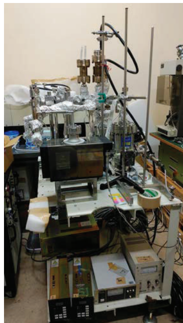
Fig. 1 A picture of the gas extraction/purification line. The line was evacuated by two turbo molecular pumps. The vacuum pressure was monitored by two ion gauges. A QMS and a sample chamber will be connected to ICF34 ports of the line.
