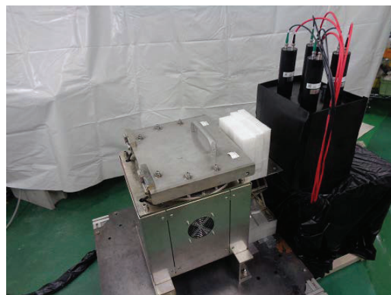
Fig. 1. The rotation machine (left), the water Cherenkov detector (right), and measurement object containing HEU (middle).
