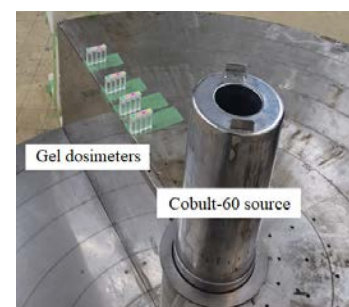
Fig. 1. Experimental setup using Cobalt-60 Gamma-ray Irradiation Facility.
