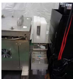
Fig. 1 The rotation machine (left), the water Cherenkov detector (right), and measurement object (middle). The center part of the object is HEU covered with lead plates.
