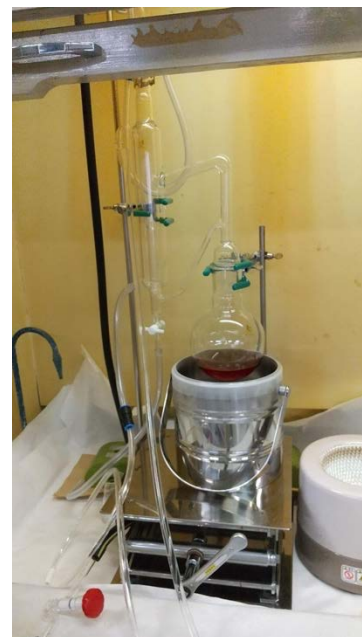
Fig. 1. Dean-Stack apparatus used for preparation of BDI and its derivatives.
