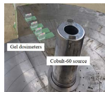
Fig. 1. Experimental setup using Cobalt-60 Gamma-ray Irradiation Facility.
