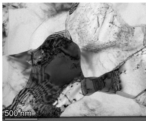
Fig. 1. Aluminum after compression at 1.5 GPa
