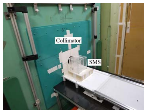
Fig. 1. Experimental setup for SMS measurements at KUR-HWNIF.
