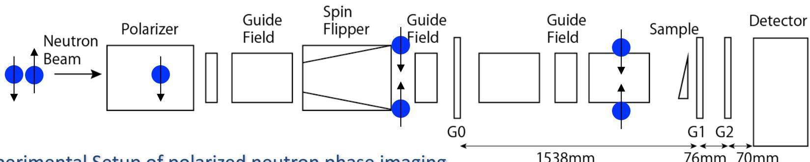
Experimental Setup of polarized neutron phase imaging
