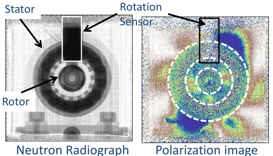
Model electric motor f=21.5Hz
