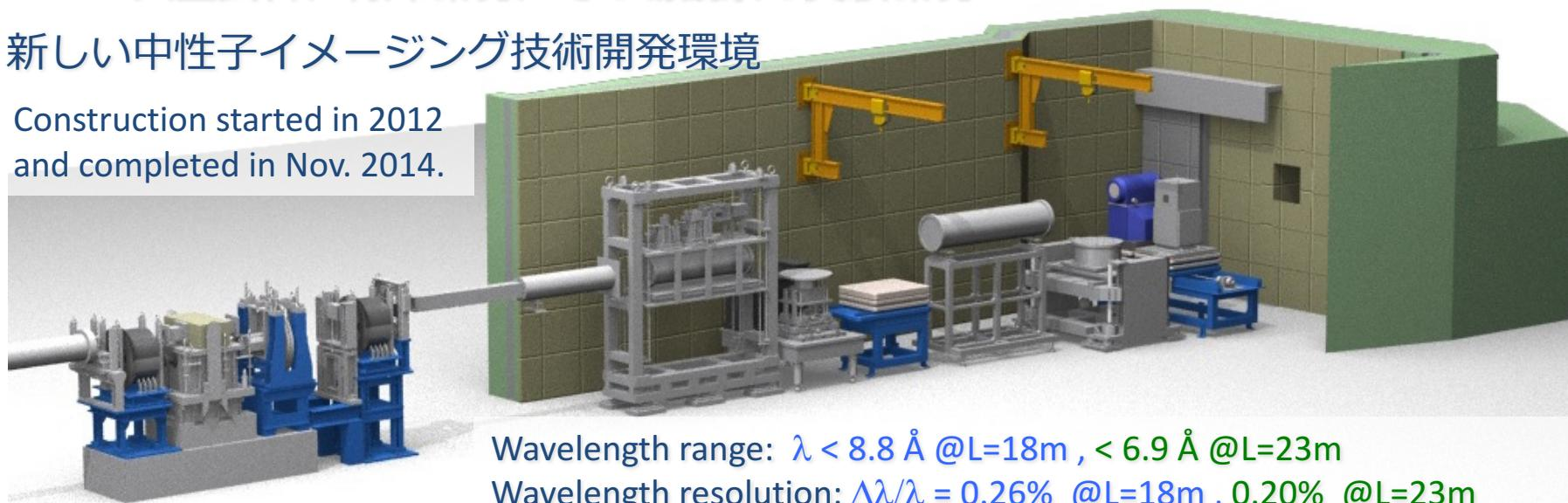
Wavelength range:  $\lambda < 8.8 \text{ \AA}$  @ $L=18\text{m}$ ,  $< 6.9 \text{ \AA}$  @ $L=23\text{m}$
