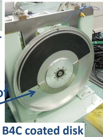
Opening angle of the disk =  $190^\circ$
