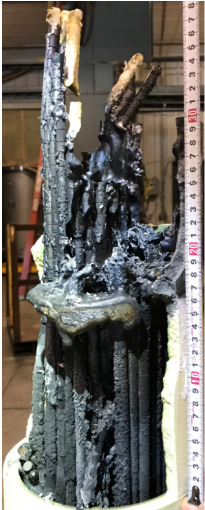
A model body for the Core Material Melting and Relocation (CMMR) study
