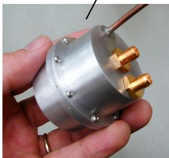
Fig. BTB fission chamber
