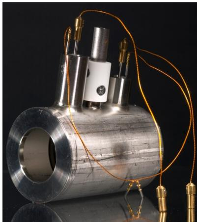
In order to keep secondary electrons with the cup a repelling voltage is applied to the polarization electrode
