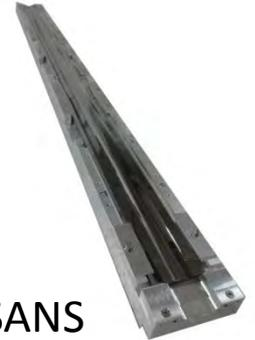
Ellipsoidal mirror (0.9m) for mf-SANS
