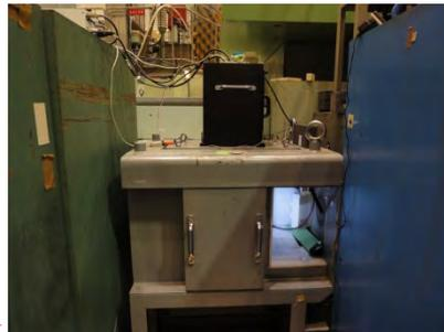
Imaging camera with <sup>6</sup>LiF+ZnS(Ag) scintillator
